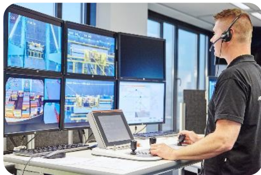
Remotely operated STS cranes
